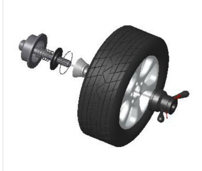
**Caution: Hold the wheel firmly during the clamping process. When inserting or removing the wheel, the wheel must not drag on the shaft.**
